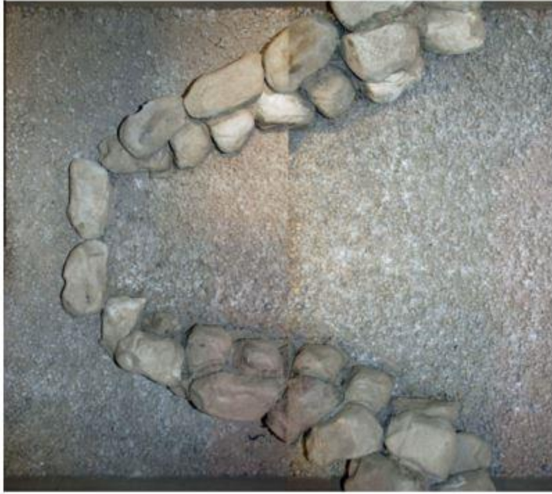
Figure 2.1 Plan view of the cross vane installed in a St. Anthony Falls Laboratory flume. Flow is from left to right. Reproduced from Kang et al. (2011).
